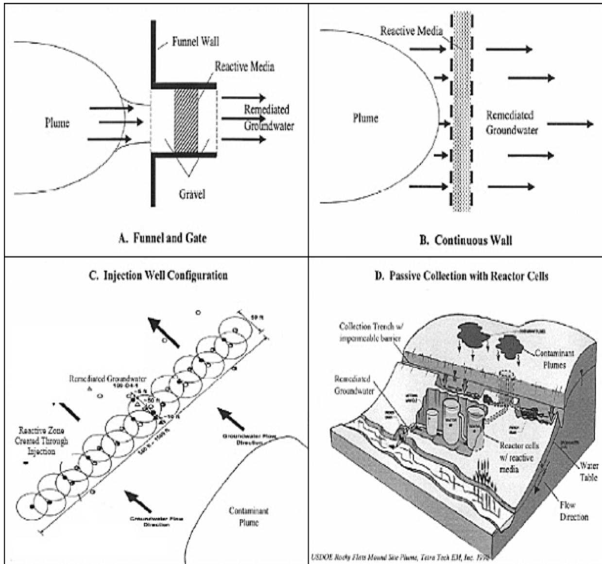
**Figure 1-2. Examples of permeable reactive barriers. (ITRC 2005)**
