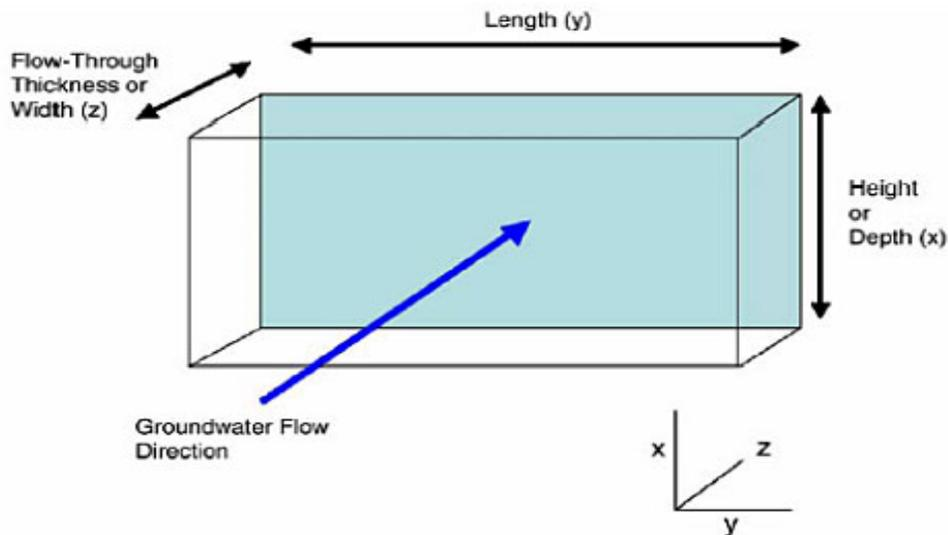
Figure 1-1. Dimensions of a permeable reactive barrier. (ITRC 2005)
