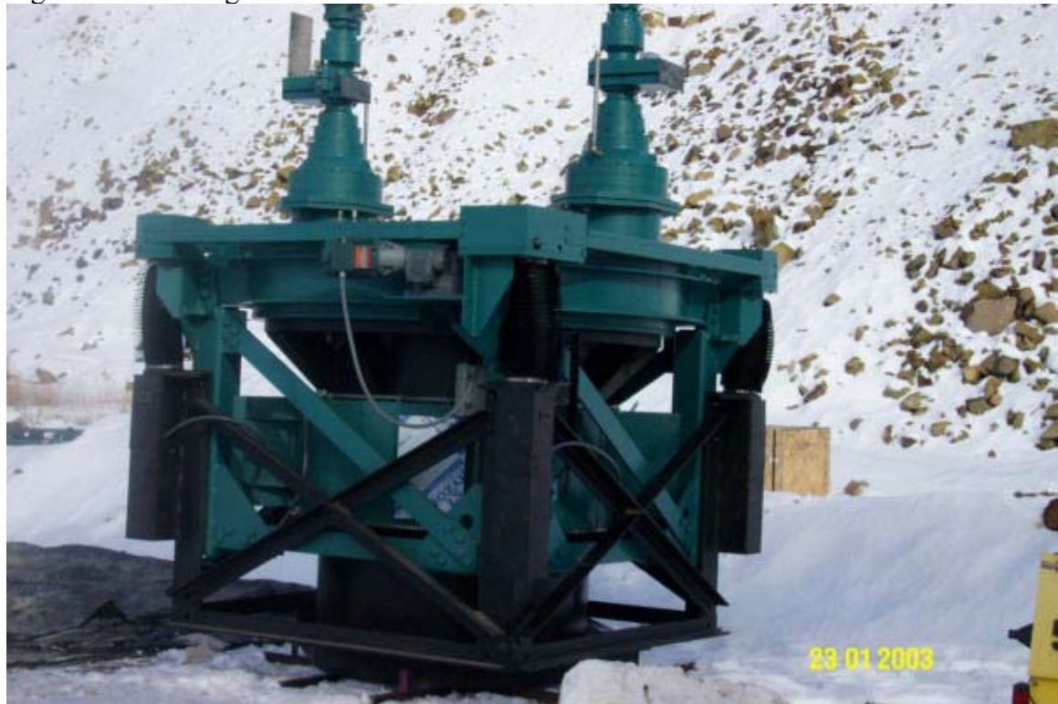
Figure 7. First Stage Clarifier Drive Mechanism
