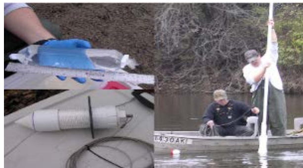
Peeper sampler (l), sampler installation (r).
