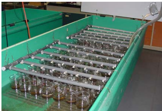
Laboratory flow through system for amphibian toxicity testing.
